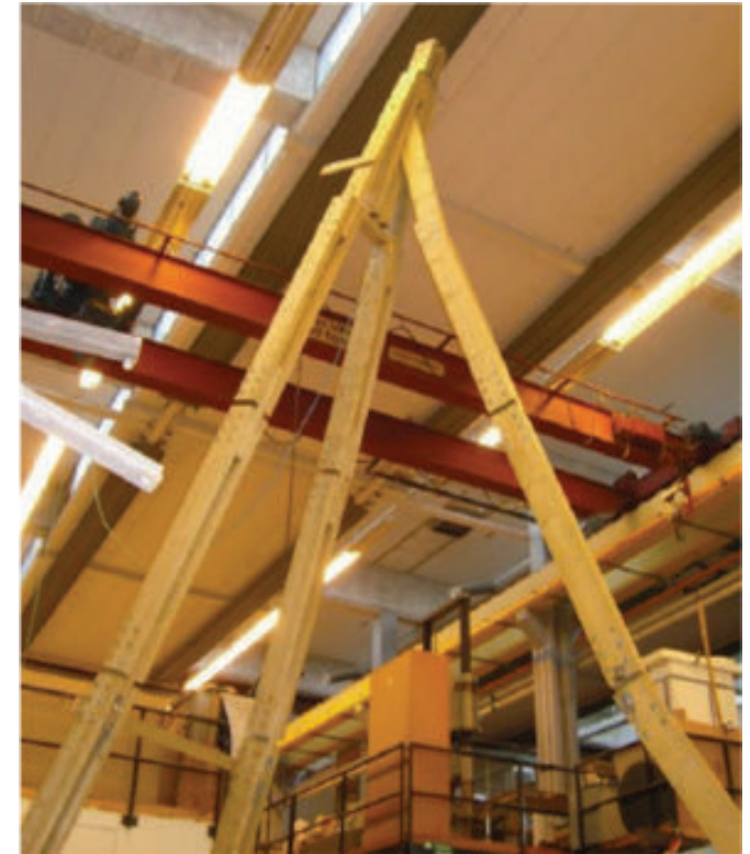
Full-scale strength testing of the Dali PowerTower at Lund University
